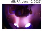
use in cutting-edge technologies. The team used high power impulse magnetron sputtering (HiPIMS) with precise timing to avoid argon inclusions, accelerating only the desired ions onto the substrate. /web/2025/05-250610-4a
