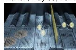
degrees, thereby creating a moiré pattern. By using different voltages applied to three electrodes, the ETH researchers subsequently produced a so-called Josephson junction, in which two superconductors are separated by a wafer-thin insulating layer, inside the twisted graphene flakes, which could have potential applications in quantum technologies.
